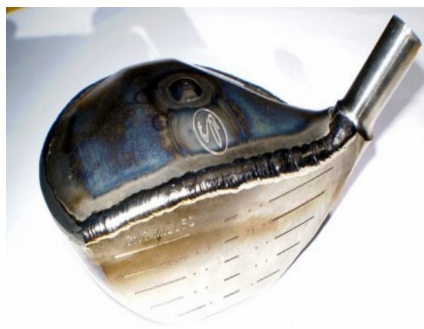
Partly machined titanium driver head donated by Robert Dunbar of Super Alloy Technologies.
